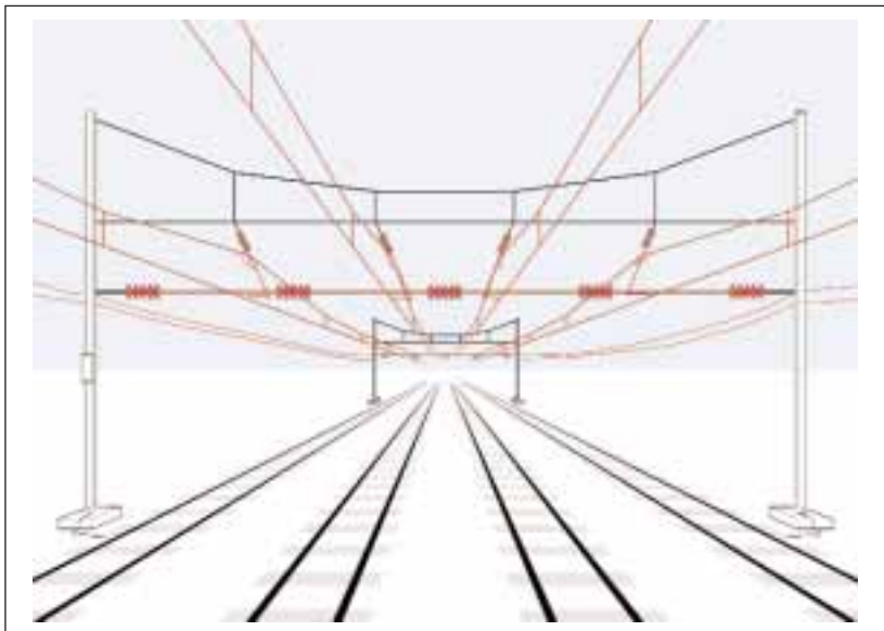
AC overhead line system
